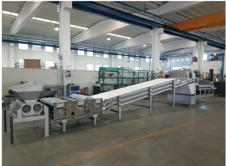
The production capacity, depending on the required configurations, may range from 50 kg / min to 500 kg / min.
